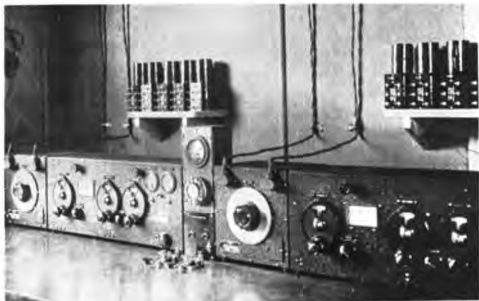
Operating Position, Pan American Airways Station "KNBI" WAKE ISLAND - 1935. Adcock Radio Direction Finder pictured on front of operations desk. Almon A. Gray Photo.
